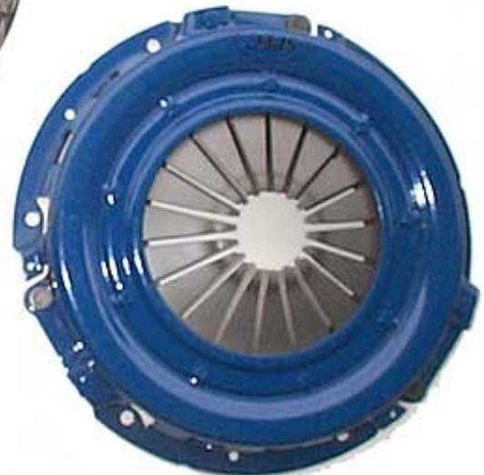
Selecting the proper clutch is a key ingredient of the T5 swap. You don't want to skimp here, otherwise you'll be doing the work all over again. We talked to the clutch experts at [SPEC \(Star Performance Engineered Clutches\)](#), and they recommended their Stage 1 clutch, PN:SF481. Their stage 1 clutch will hold 300 horsepower with no problems, yet allow for chatterless engagement and low rpm driveability. At about \$159, including throwout bearing and alignment tool, the price is right too.
