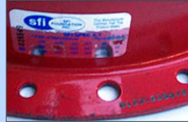
The SFI certification is only good for two years. Technically this means you need to replace the bellhousing every two years. This baffles us since this isn't a component that wears out. Furthermore we've never heard of a tech official checking the date on the tag.
