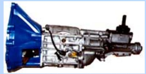
Seek out a T5 from a V8 car, ideally a Mustang. The 1983-1989 V8 T5's are rated at 265 lb.ft. of torque, while the 90-93 T5's are rated good to 300lb.ft. Typically these can be had for \$200-600 used. A new T5 will run about \$1000.
