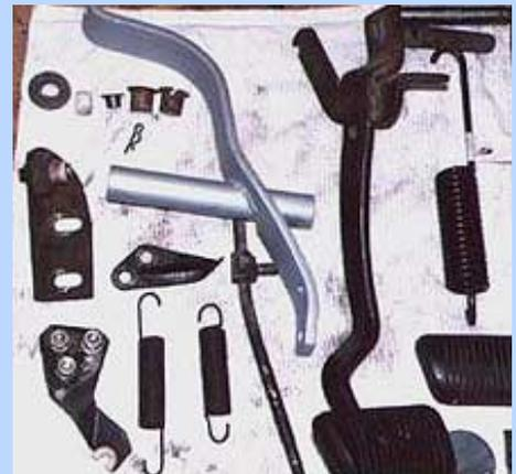
Converting an early Ford from automatic to manual requires rounding up the original clutch activation parts. This can be tough, the best bet is to find a wrecked four-speed car and take everything. Shown here are parts from an early Mustang, including the z-bar
