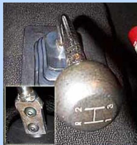
You can maintain the stock look by modifying the early shifter. We hacked off the 3spd/4spd lower bracket and welded on a metal tab. Drill two 3/8" holes to match the T5 shifter nub. Slip the stock boot over it and no one can tell from the inside that you've got an extra gear!
