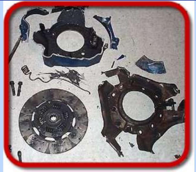
Send in the bomb squad: The entire aftermath of this clutch explosion can't even be seen in this photo. Shrapnel poked a hole in the hood, pinched a header collector in half, ripped the accelerator pedal right off the firewall, destroyed the shock tower brace, severed the main engine harness, and knocked out a freeze plug in the back of the block. It's amazing the driver wasn't injured.
