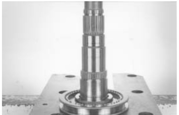
12.- Using a special tool or press, install the 1 st & 2 nd synchronizer, as indicated.
