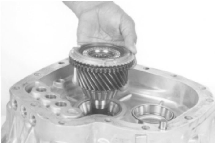
69.- Remove the input shaft, as indicated.
