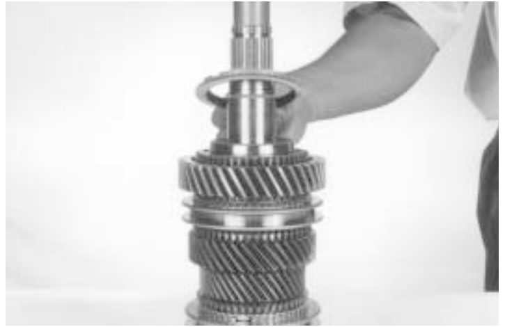
46.- Remove the reverse gear blocking ring, as indicated.
