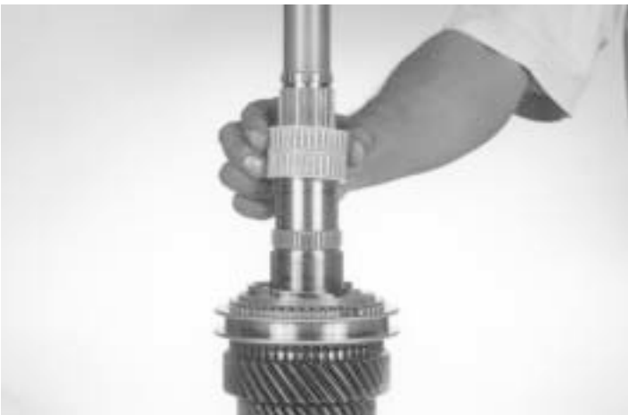
49.-Remove the needle bearing from first gear, as shown.
