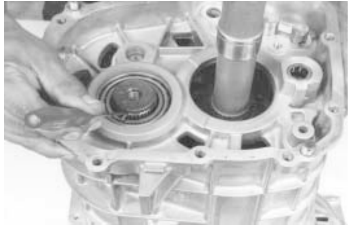
31.- Remove the transmission case from the clutch housing, as indicated. Use a hook to hold the bearing cone to avoid interference with the cluster gear.
