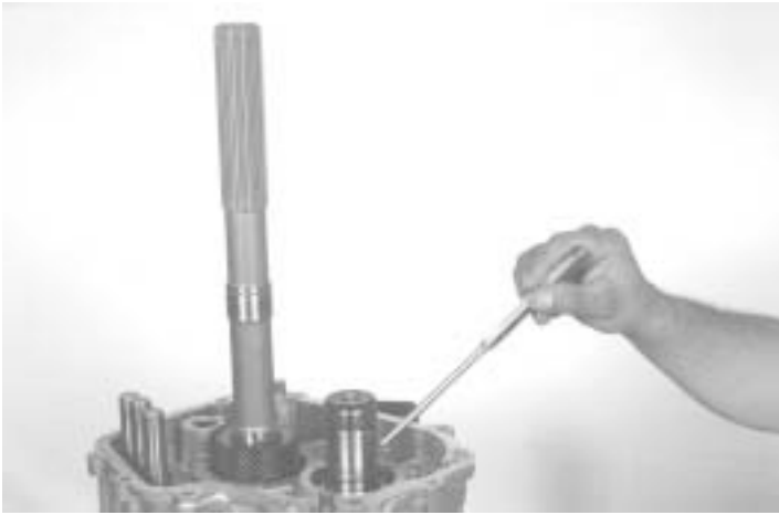
86.- Using a magnet install the locating ball, as indicated.
