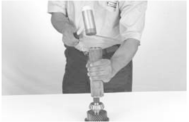
52.- Using a special tool or press, install input shaft bearing cone, as shown.
