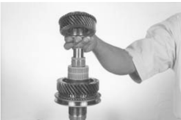
23 .- Install the third speed gear, as indicated.
