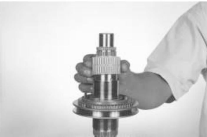
17.- Install the second gear needle bearing, lubricate with the recommended transmission fluid.
