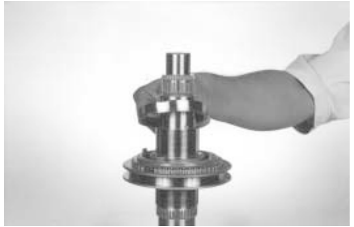
16.- Install the second gear synchronizer inner cone, as indicated.
