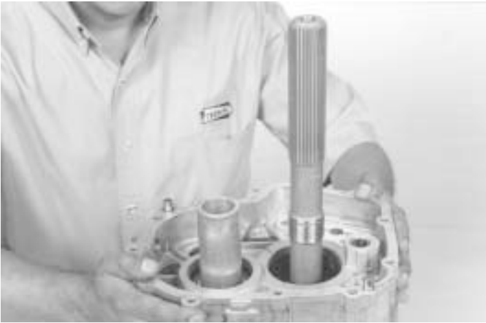
78.- Install the transmission case, as shown.
