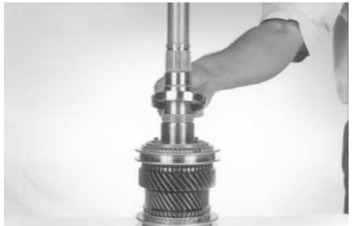
30.- Install the inner first gear synchronizer cone, rotate the inner cone till it is seated, as indicated.
