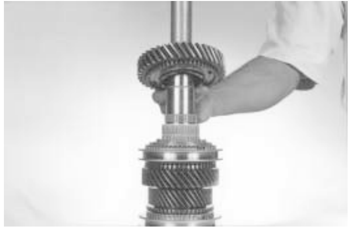
32.- Install the first speed gear, rotate the gear to align gear slots with the inner cone tabs.
