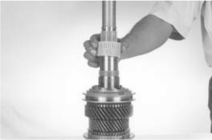
31.- Install the first gear needle bearing lubricate with the recommended transmission fluid.
