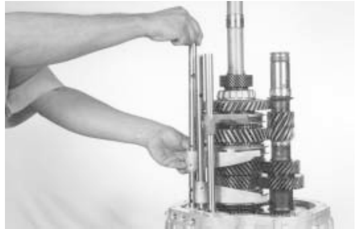
35.-Remove the 1st. & 2nd, fork and shift rail, as indicated.
