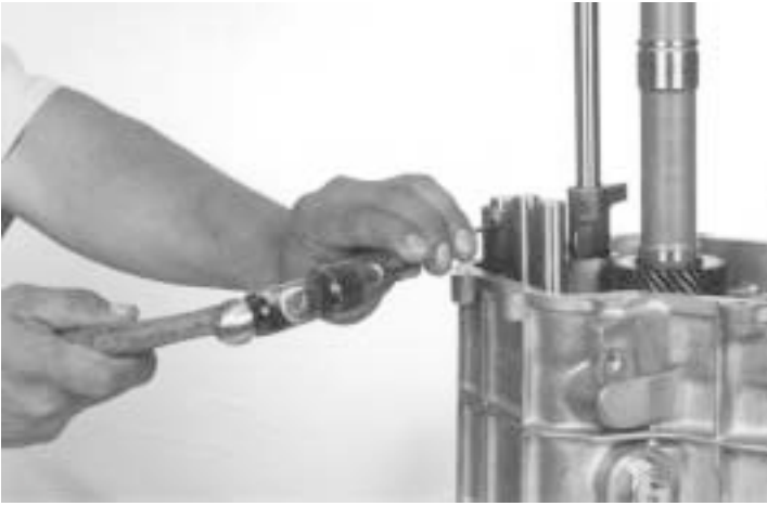
19.- Using a 5/32-inch drift and hammer, drive out the split pin then remove the 1st & 2nd shift gate.
