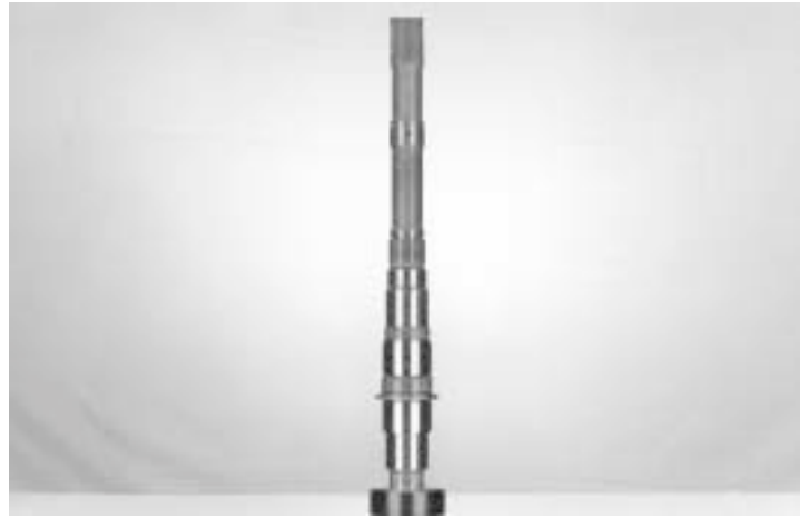
10.-Install the mainshaft in a support or vise with soft jaws or wood, shaft front facing up, as indicated.
