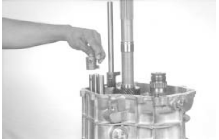
91.- Install the 1 st & 2 nd shift finger, as shown.
