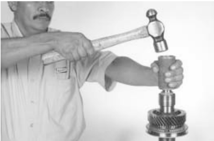
21.- Using a special tool or a press, install the spacer, thrust washer and second speed gear, as shown.
