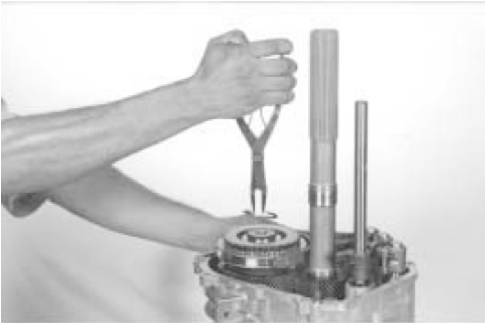
15.-Using a snap ring plier, remove the snap ring of the fifth gear assembly, as shown
