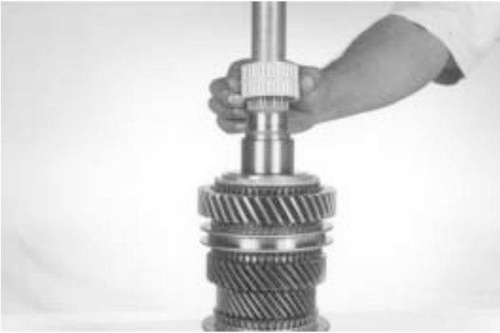
45.- Remove reverse gear needle bearing, as shown.
