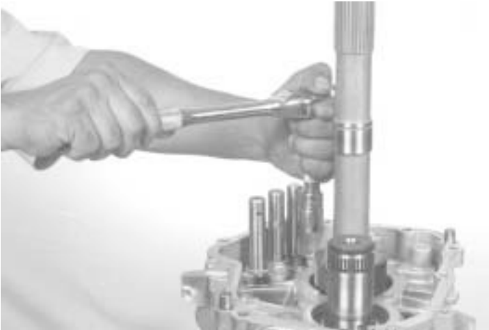
25.-Remove the two bolts from the shift interlock plate, as shown.
