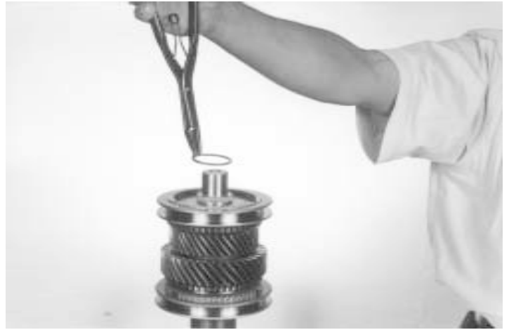
26.- Using a snap ring plier, install the 3 rd & 4 th hub snap ring, as shown.
