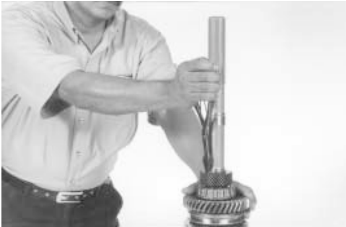
42- Remove the retaining ring above fifth gear, as shown.
