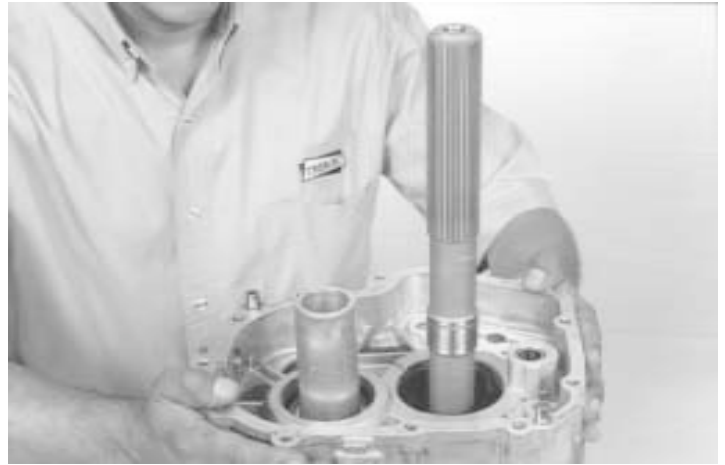
62.- Install temporarily the transmission case, as shown.
