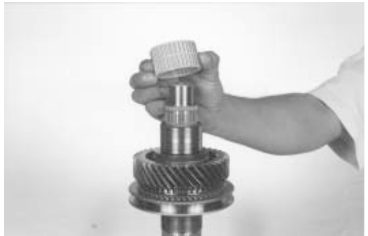
22.- Install the third gear needle bearing, lubricate with the recommended transmission fluid, as shown.
