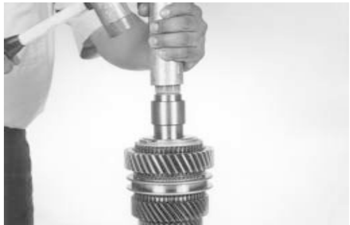
36.- Use a special tool or a press to install, as indicated.
