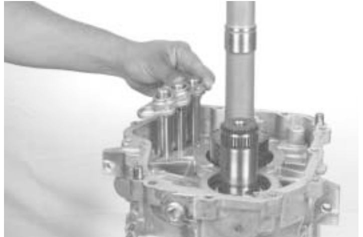
26.- Remove the shift interlock plate, as indicated
