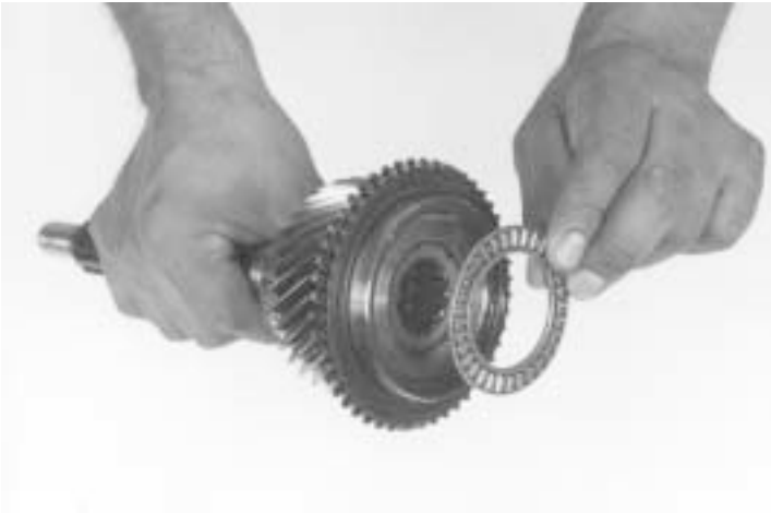
71.- Remove the axial bearing, as shown.
