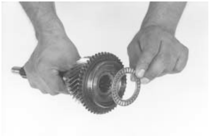
54.- Install the input shaft bearing, as shown.
