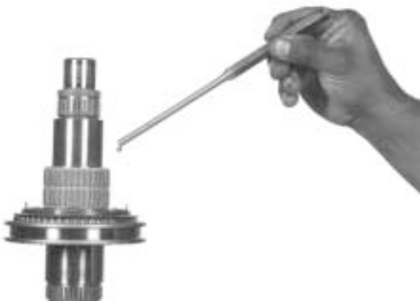
60.- Remove the locating ball, as shown.
