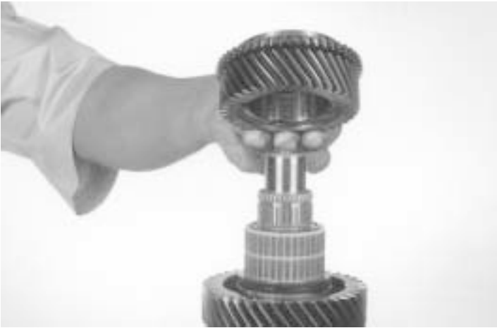
57.- Remove the third speed gear, as shown.
