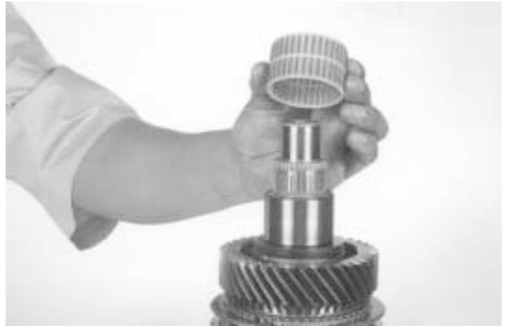
58.- Remove the third gear needle bearing, as indicated.
