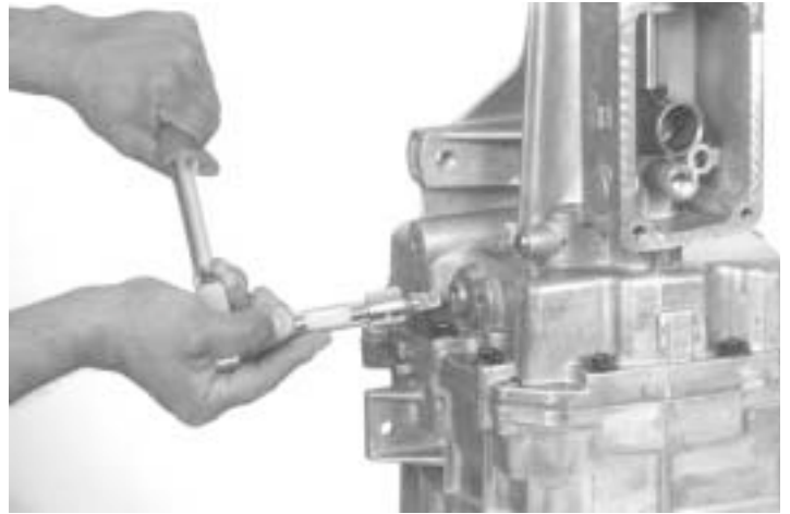
8.-Remove the fill plug, as indicated
