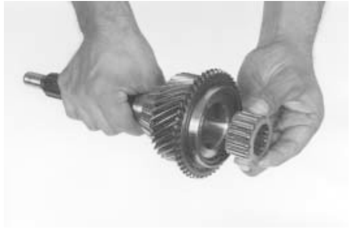
72.- Remove the input shaft needle bearing, as shown.
