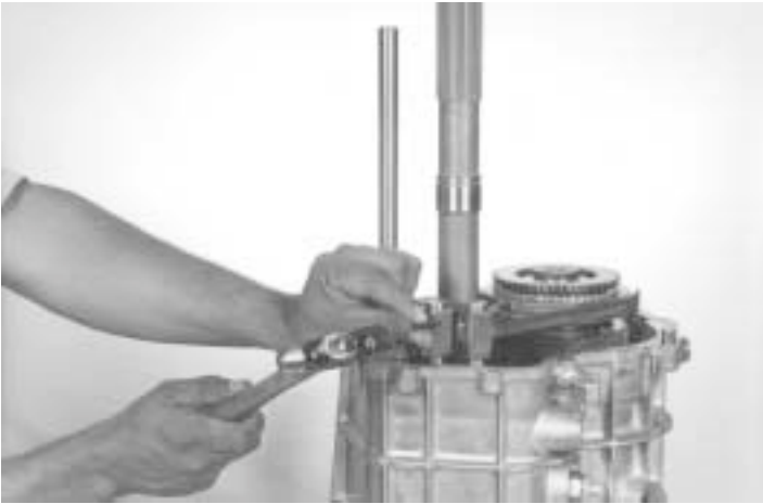
96.- Using a 5/32-inch drift and hammer, install the 5 th fork pin on the shift rail.
