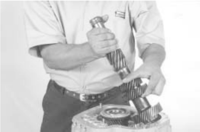
57.- Install the countershaft, as indicated.
