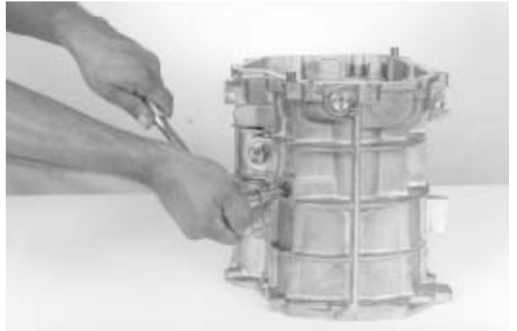
79.- Remove the reverse idler shaft bolt. Remove and discard the seal, as indicated.
