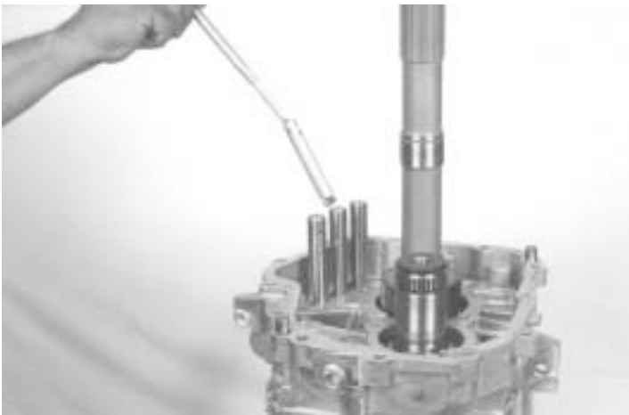
82.- Using a magnet, install the interlock pins, as indicated.
