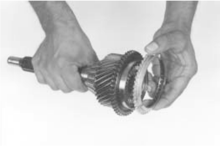
55.- Install the synchronizer blocking ring, as indicated.
