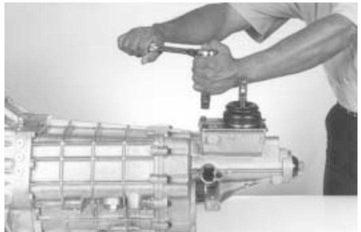
113.- Install the four bolts and tighten to the recommend torque, as indicated.
