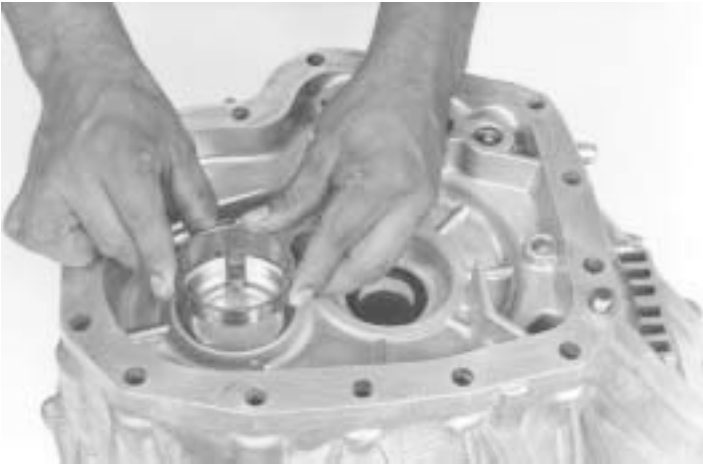
49.- Install the front countershaft bearing cup, as indicated.
