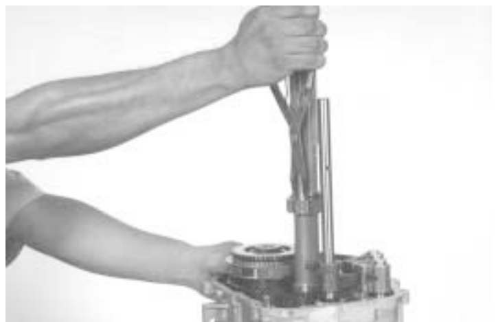
12.- Using a snap ring plier, remove the sensor speedometer snap ring, as indicated.
