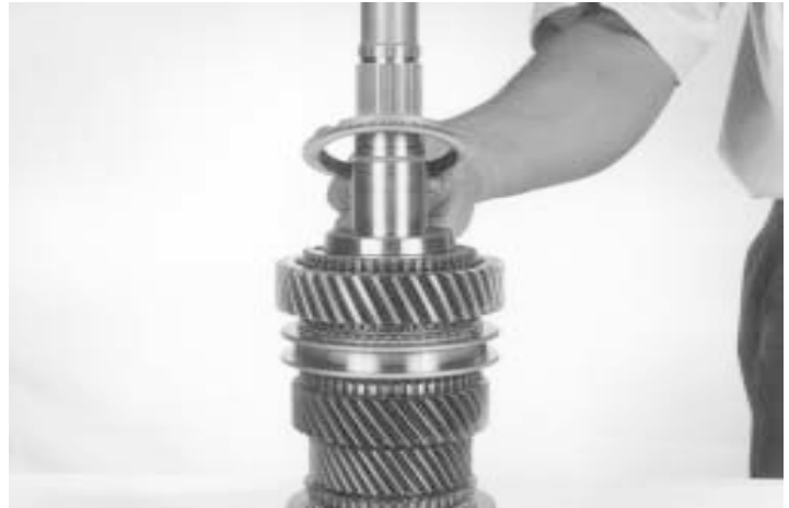
34.-Install the reverse gear blocking ring, as indicated
