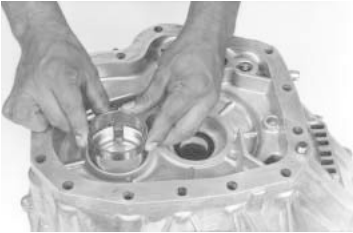
76.- Remove the bearing cup, from the counter shaft, as shown.
