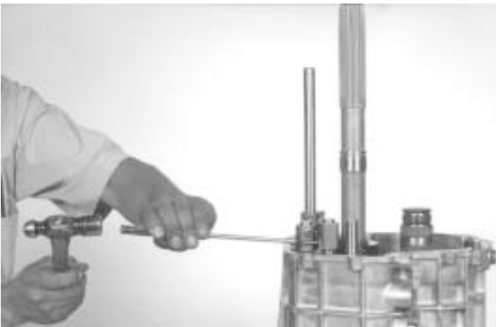
94.-Using a 5/32-inch drift and hammer, install the 3 rd & 4 th gate pin on the shift rail.
