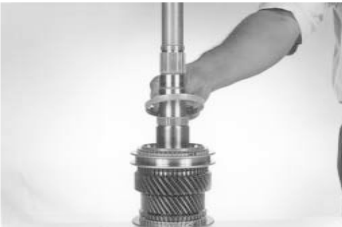
29.- Install the outer first gear synchronizer cone, as shown.
