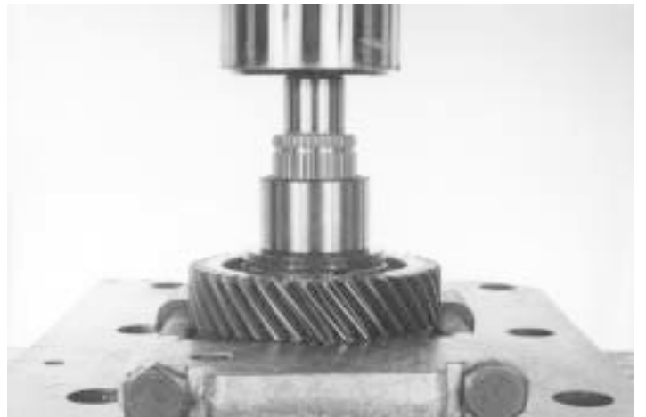
59.- Using a special tool or a press, remove the spacer, thrust washer and second speed gear
