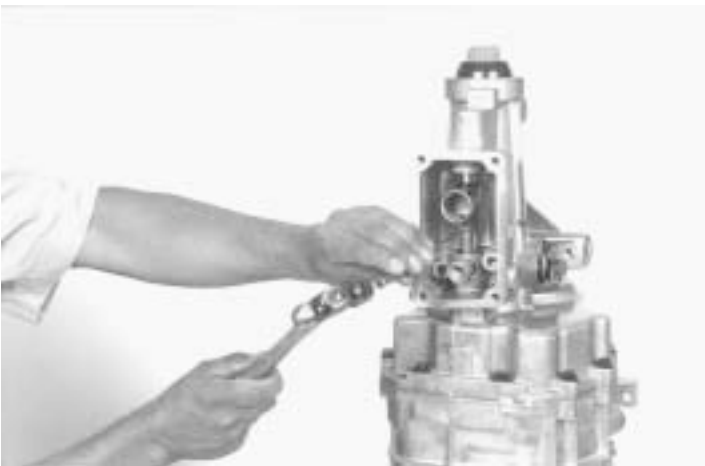
106.-Using a 5/32-inch drift and hammer, install the off set lever pin, as shown.
