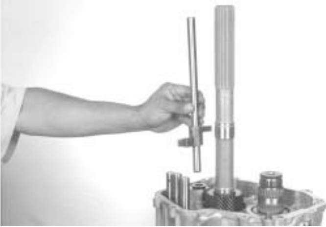
90.- Install the main shift rail, as indicated.
