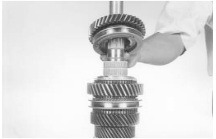
38.- Install reverse gear, rotate gear to align the gear slots with the inner cone tabs.
