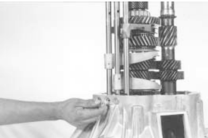
76.- Install the three detent plugs, as shown
