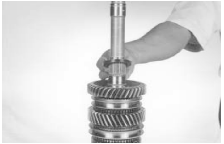
40.- Install the thrust washer. Be sure to align the slot in the washer with the ball.
