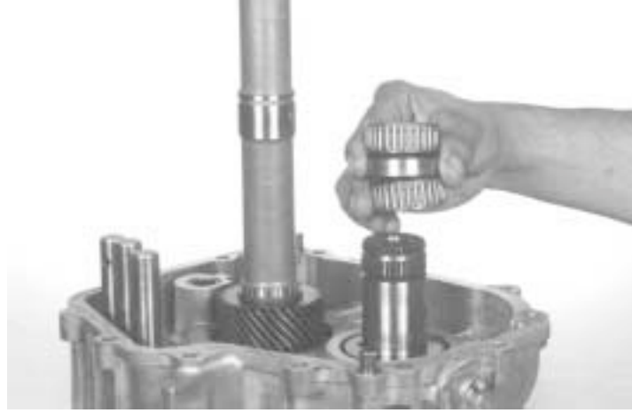
22.-Remove the two needle bearings and the spacer, as indicated.
