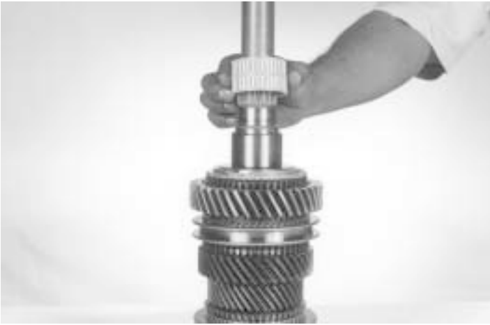
37.-Install reverse gear needle bearing, lubricate with the recommended transmission fluid,as shown.
