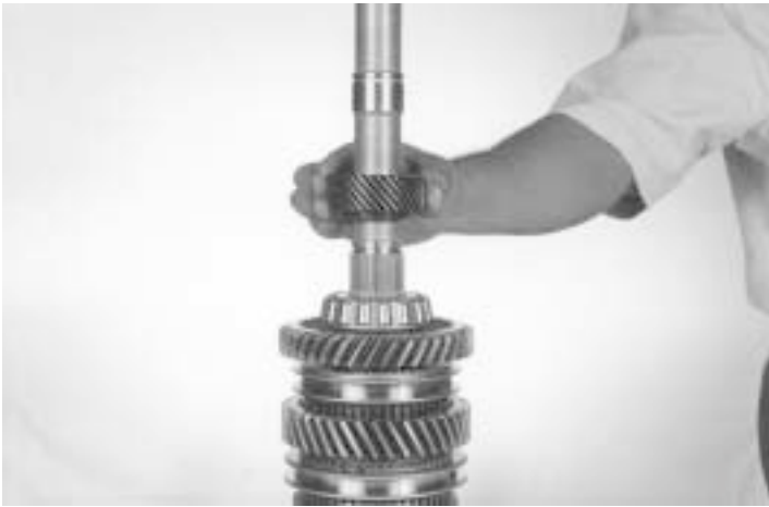
43.- Intalll the 5 th speed gear, as shown.
