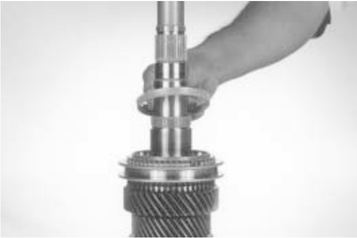
51.- Remove the outer first gear synchronizer cone, as shown.
