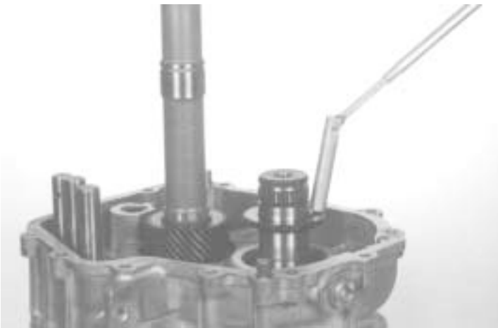
23.- Using a magnet, remove the ball, as shown.
