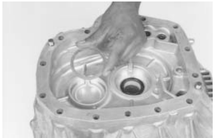
48.- Install the appropriate shims to achieve the proper end play, this total gives you a shim pack thickness to start the end play measurement.
