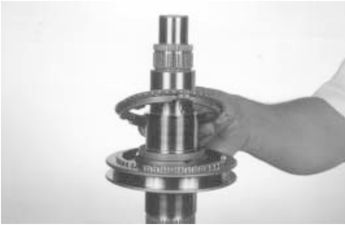
64.- Remove the second speed gear synchronizer blocker ring, as shown.
