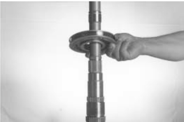
11.- Install 1 st & 2 nd synchronizer assembly, as shown
