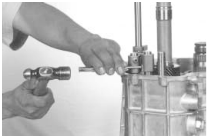
18.- Using a 5/32-inch drift and hammer, drive out the split pin, then remove the 3 rd & 4 th shift gate, as indicated
