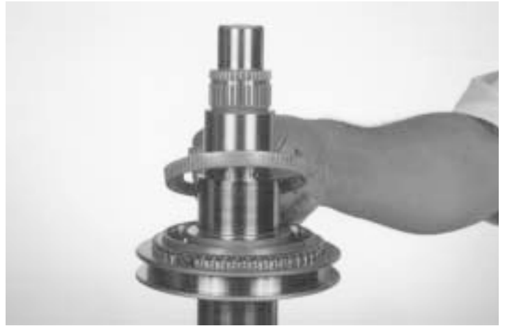
63.- Remove the second speed gear synchronizer outer cone, as indicated.
