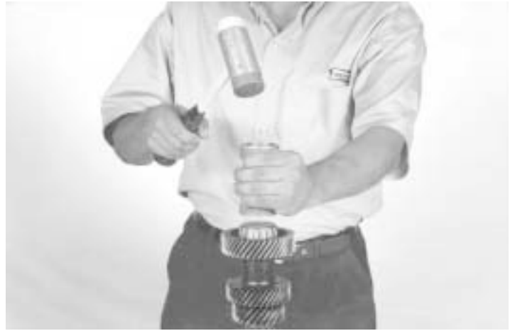
46.- Using a special tool or press, install the countershaft bearing cone, as shown.
