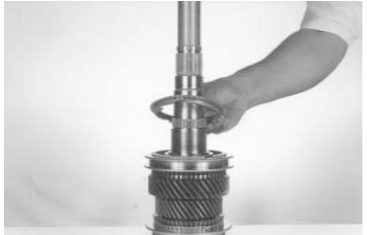
28.- Install the first gear synchronizer blocking ring, align the blocking ring tabs with the synchronizer assembly. Rotate mainshaft with synchronizer up, as shown.
