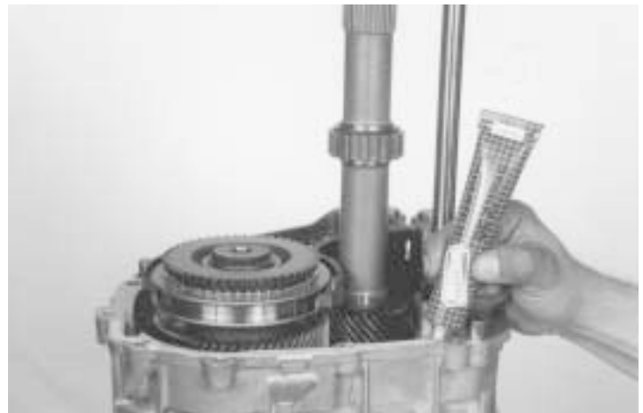
101.- Clean the mating surfaces of the transmission main case, and the extension housing. Apply a bead of silicone rubber to the sealing surface of the transmission case.
