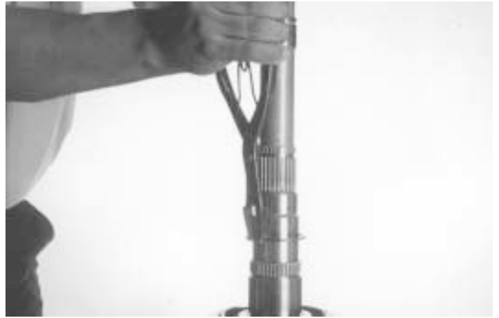
65.- Using a snap ring pliers, remove the 3 rd & 4 th hub snap ring, as indicated.
