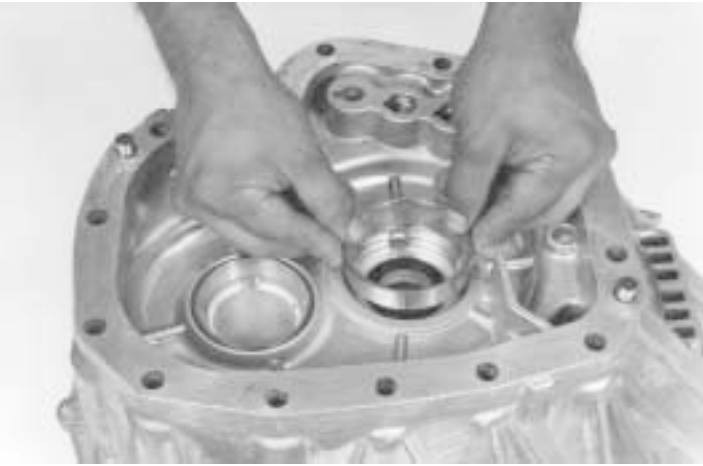
51.- Install the front input shaft bearing cup, as indicated.
