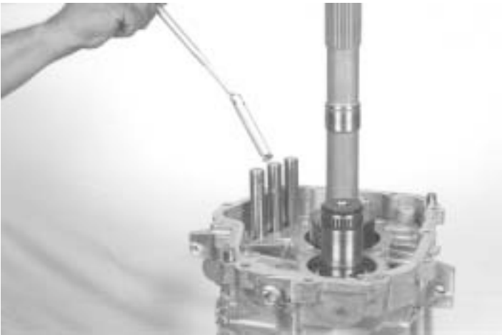
27.- Using a magnet, remove the interlock pins, as shown.
