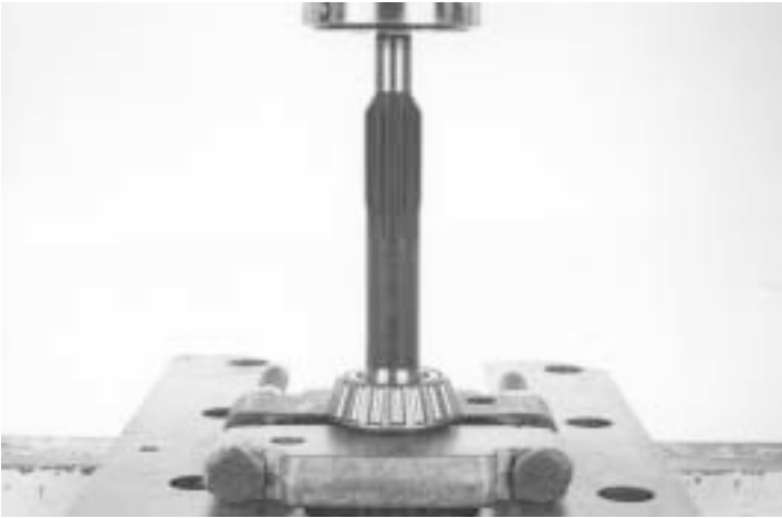
73.- Using a special tool or a press, remove the cone bearing from the input shaft, as shown.
