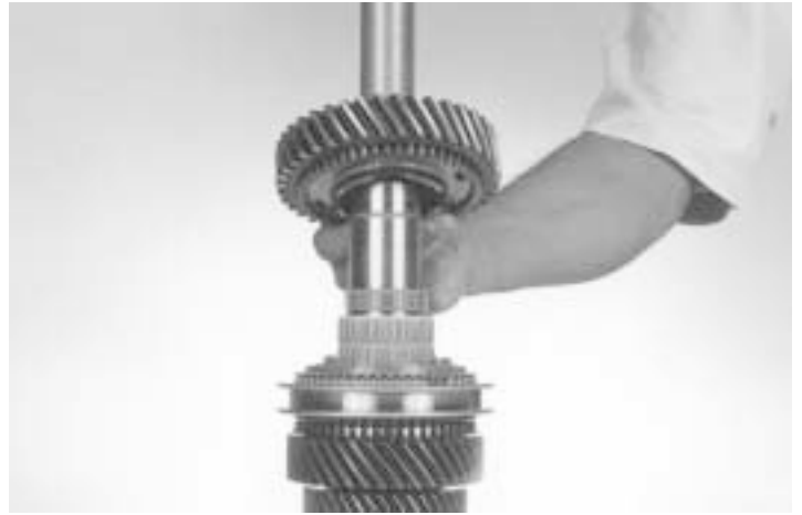
48.- Remove the first gear, as indicated.
