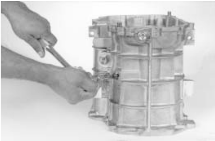
3.- Install a new seal and the reverse idler shaft bolt, as shown.
