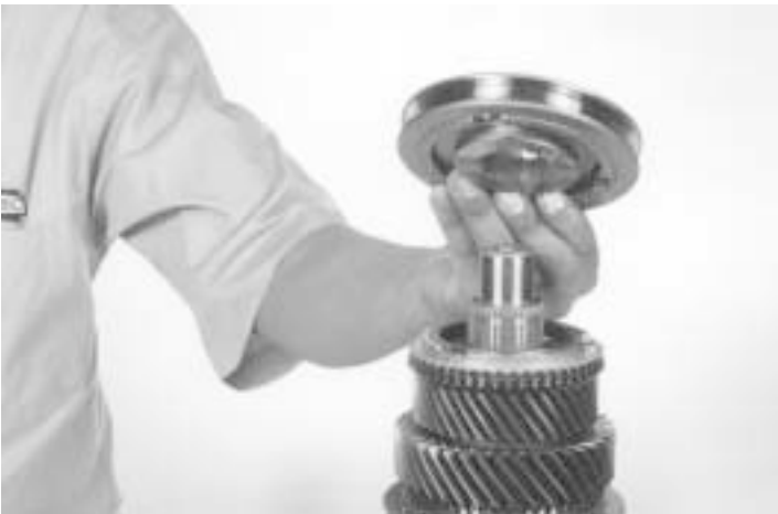
55.- Remove the 3rd & 4th speed synchronizer, as shown.
