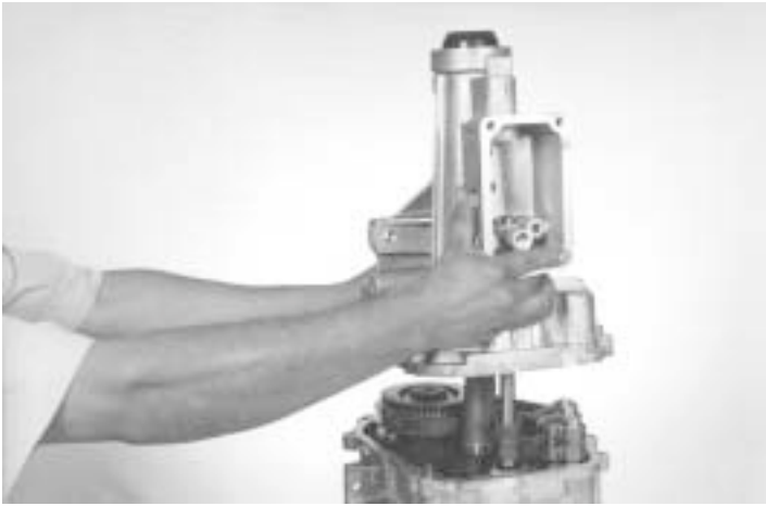
102.- Install the extension housing and at the same time install the gear shift off-set lever.
