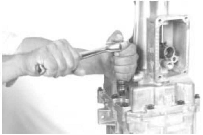
103.- Install the (12) bolts and tighten to the recommended torque, as indicated.
