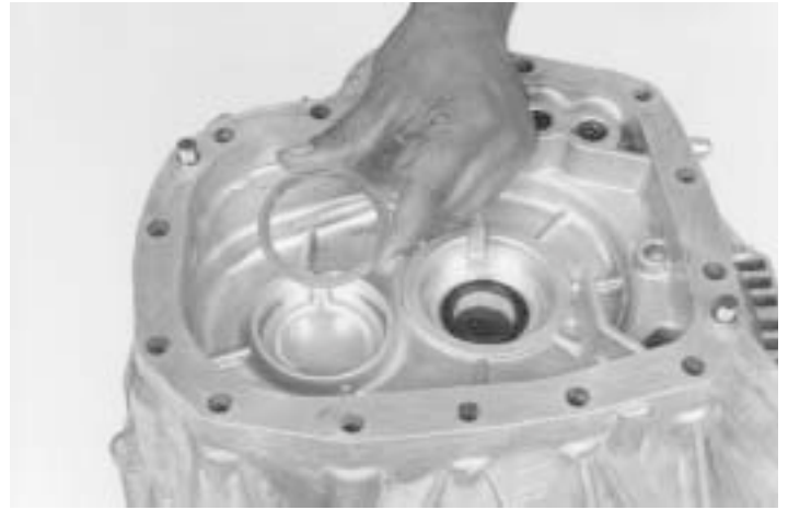
77.- Remove the bearing shim, from the counter shaft, as indicated.
