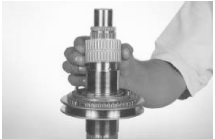
61.- Remove the second speed gear needle bearing, as indicated.
