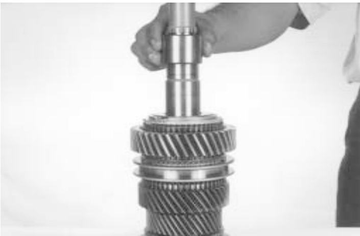
35.-Install the reverse gear bearing spacer, as shown.
