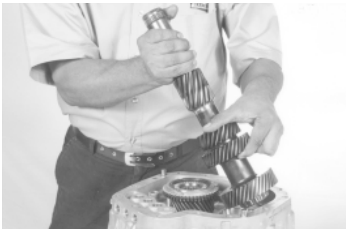
67.- Remove the countershaft, as shown.
