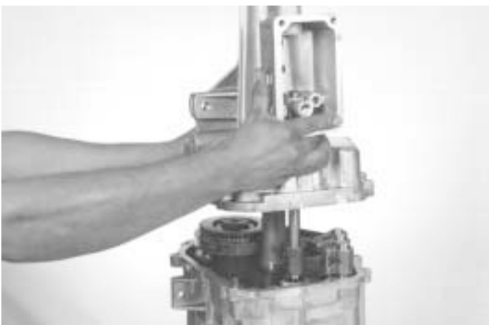
11.-Remove the assembly extension housing, as shown.
