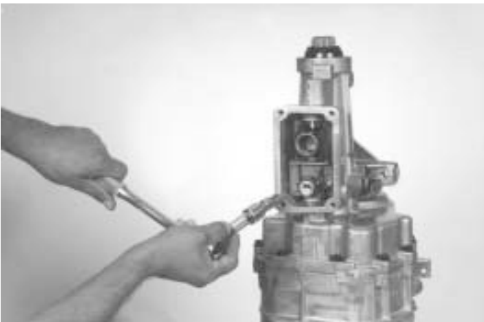
5.- Using a 1/4" socket, remove the bolts, as shown.
