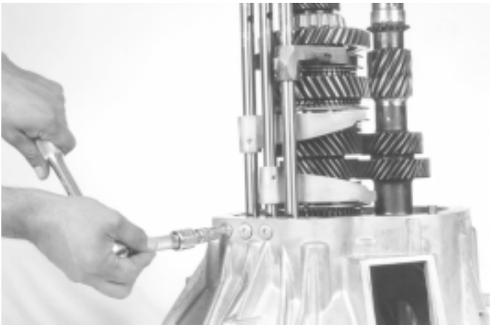
32.- Remove the three detent plugs, as shown
