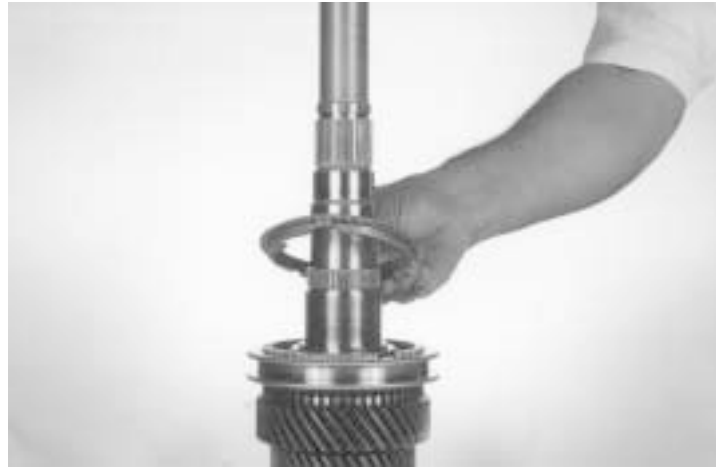
52.- Remove the first gear synchronizer blocking ring, as indicated.
