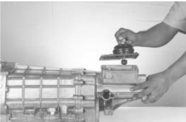
112.- Install the control turret assembly, as shown
