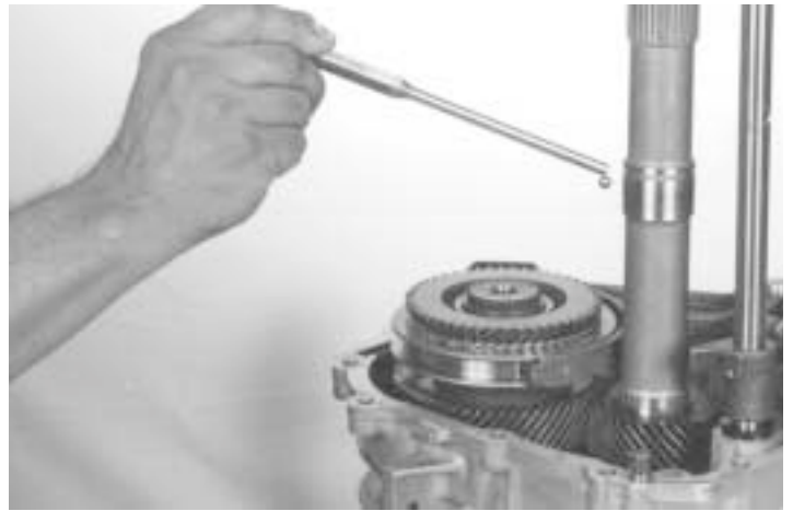
14.-Using a magnet, remove the ball, as indicated.
