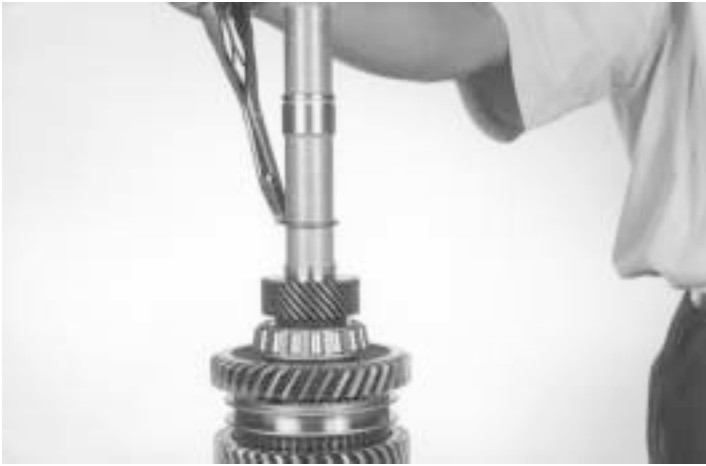
45- Using a snap ring plier, install the 5 th gear snap ring, as indicated.
