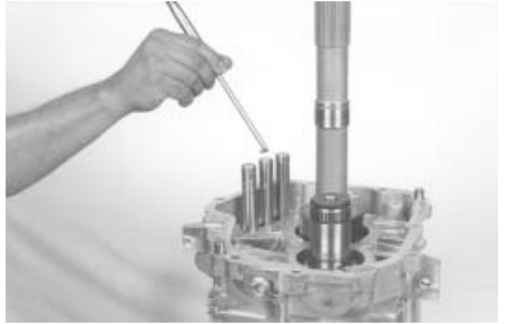
81.- Using a magnet, install the lock pin in the center rail, as shown
