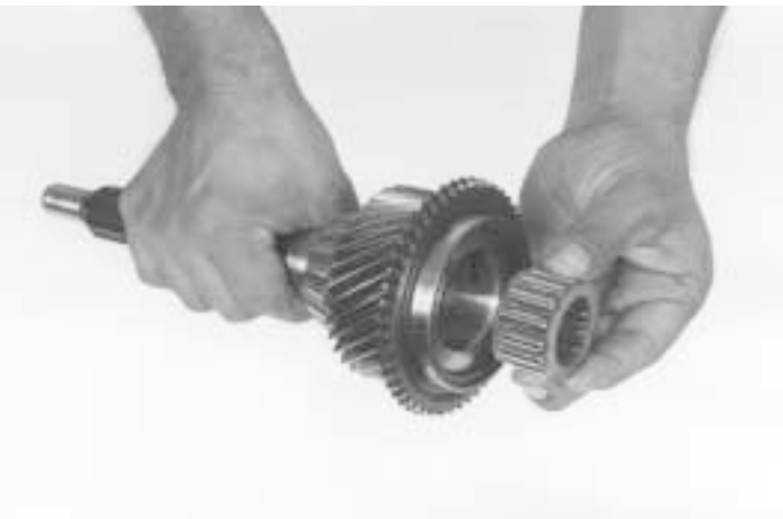
53.- Install the input shaft needle bearing, as indicated
