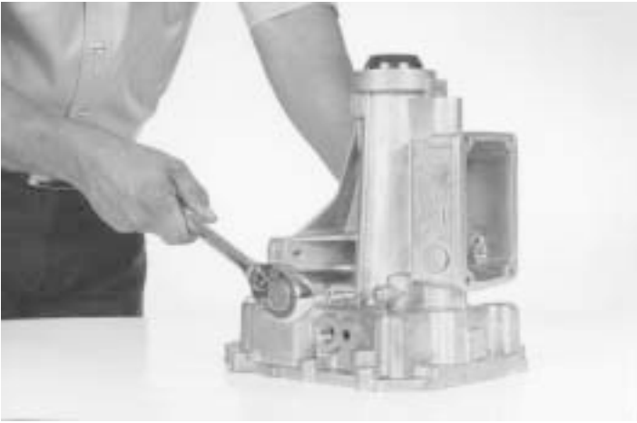
9.-Install the fifth & reverse gear lockout bolt, as shown.
