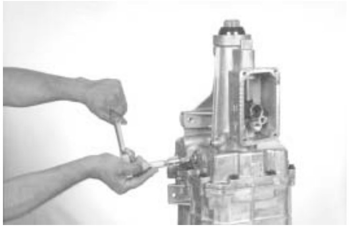
105.-Using a 10 mm. socket tighten to the recommended torque.
