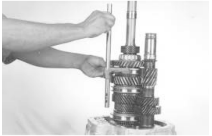
67.- Install the reverse & 5th rail, as indicated.
