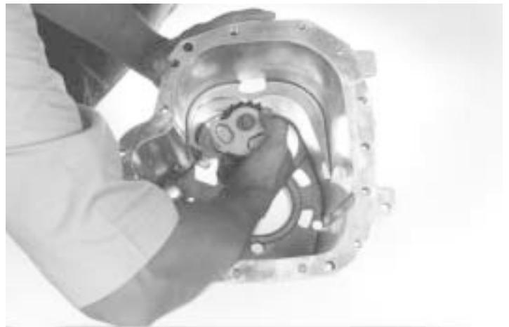
81.- Remove the reverse gear, the shaft and support shaft, as indicated.
