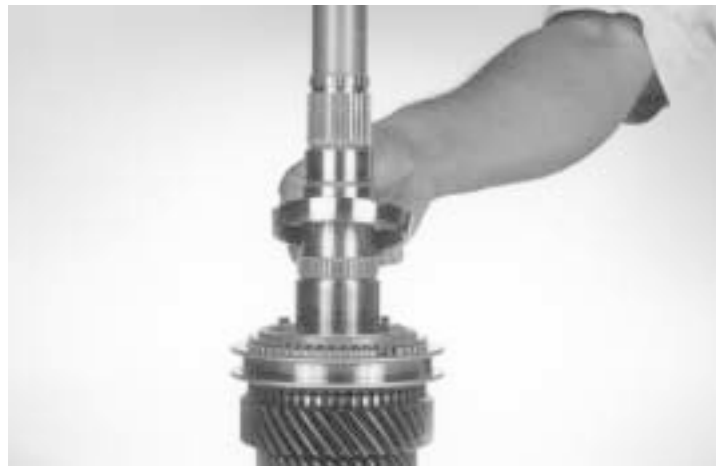
50.- Remove the first gear synchronizer inner cone, as indicated.
