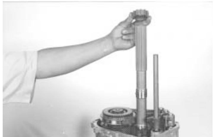
99.- Install the speedometer sensor, as indicated.
