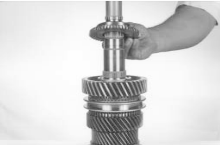
33.- Install the reverse clutch cone, as shown.
