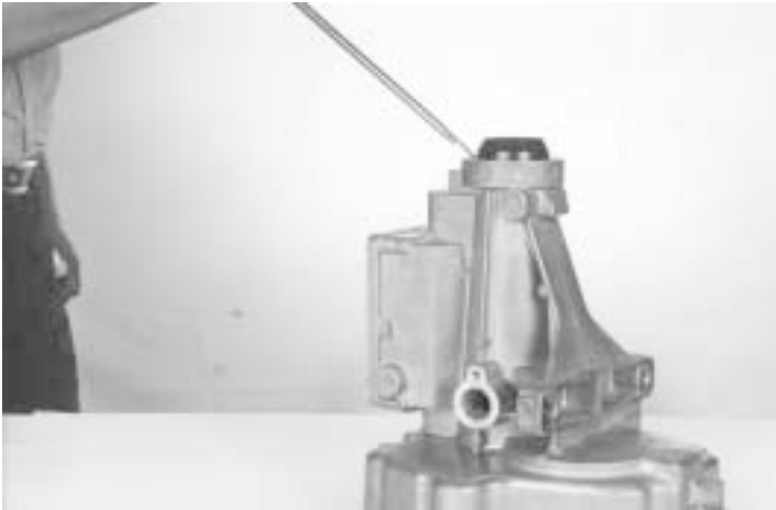
88.- Using a special tools, remove the extensión housing fluid seal, as shown.
