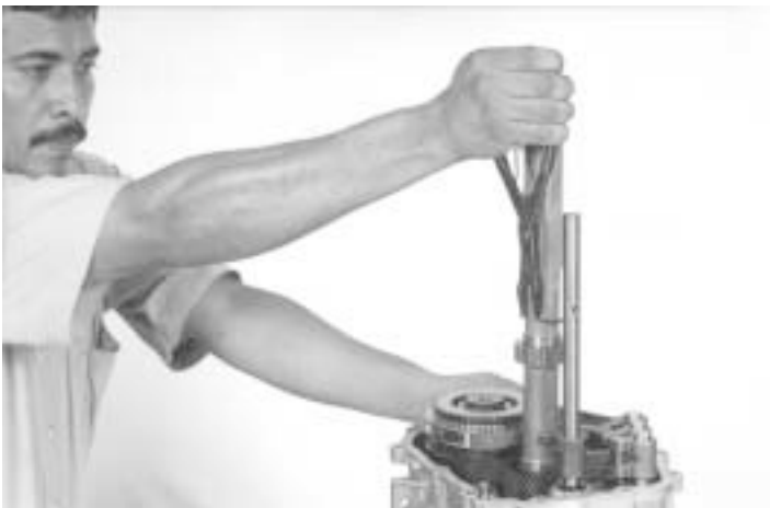
100.-Using the snap ring plier, install the sensor snap ring, as indicated.
