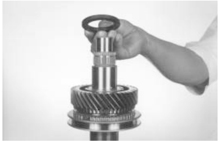
20.- Install the thrust washer, as indicated.
