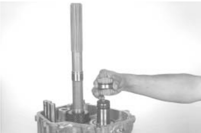
88.- Install the two needle bearing and spacer, as indicated.
