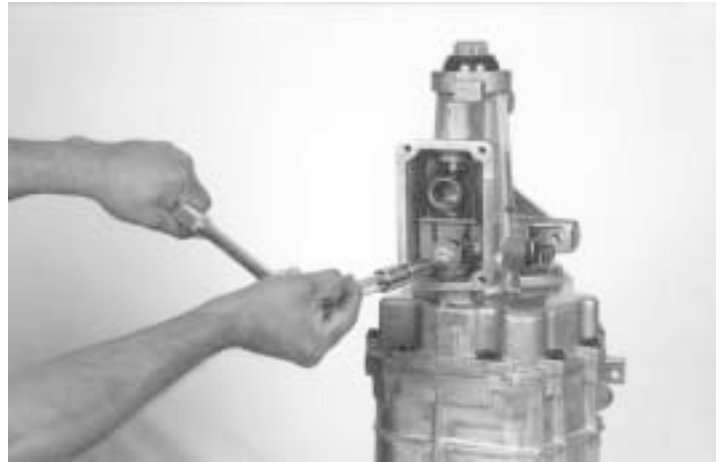
4.- Rotate the transmission to a vertical position, and remove the bolt and washer, that hold the spring and plate.
