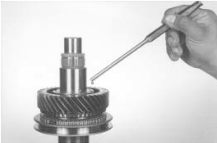
19.- Install the locating ball, as shown.
