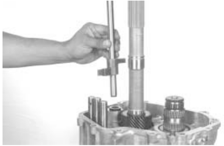
20.- Remove the main shift rail, as indicated.
