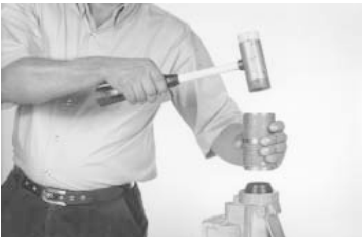
5.- If previously removed, install the extension seal with the proper seal driver.
