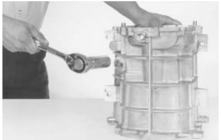
4.- Install the reverse switch, as indicated.
