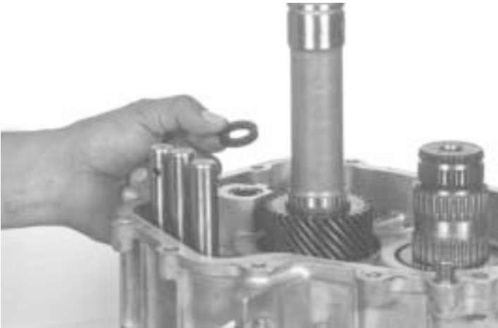
21.-Remove the plastic spacer, as shown.
