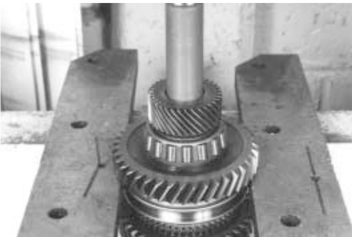
43- Using a special tool or a press, remove the fifth gear, the spacer, the output shaft bearing and reverse gear from the output shaft bearing.
