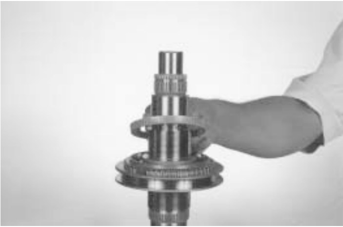
15.- Install the second gear synchronizer outer cone, as shown.
