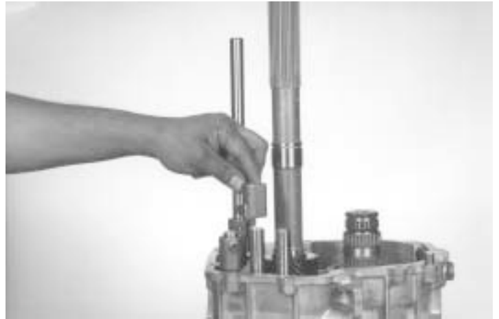
93.- Install the 3 rd & 4 th shift finger, as shown.
