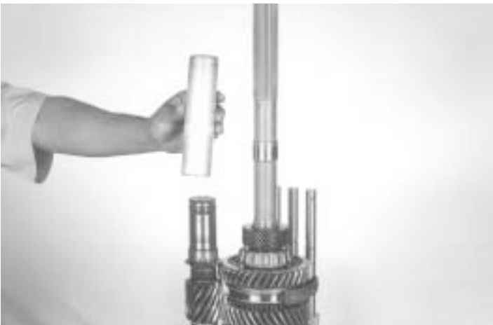
59.-Install a tube as a guide when installing the counter shaft bearing cone, as indicated.
