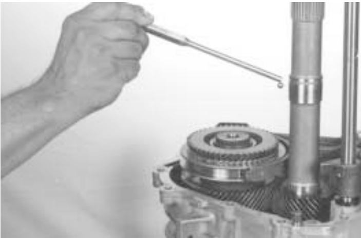
98.- Install the ball for speedometer, using a magnet, as shown.
