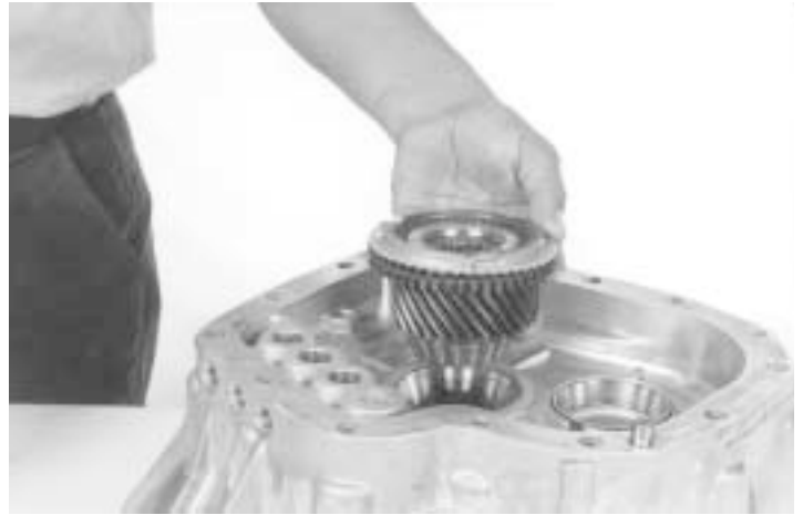
56.- Install the input shaft, as shown.
