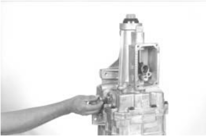
104.- Install the fill plug, as shown.
