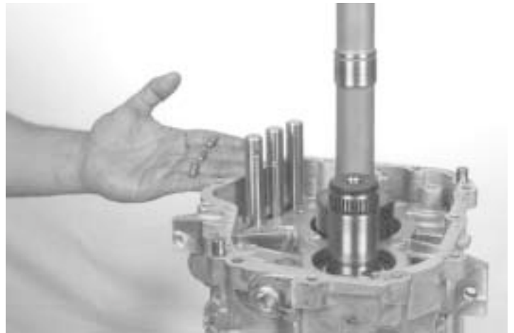
28.-Position the interlock, and lock pin on the center rail, two between the rails.
