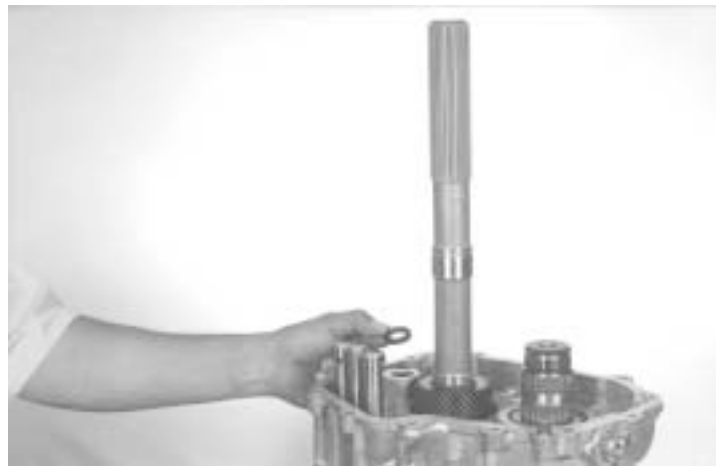
89.- Install the plastic spacer, as shown.
