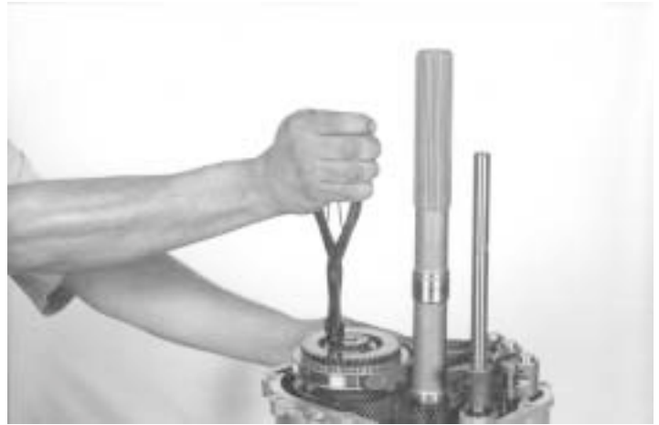
97.-Using a snap ring plier, install the 5 th gear snap ring, as indicated.
