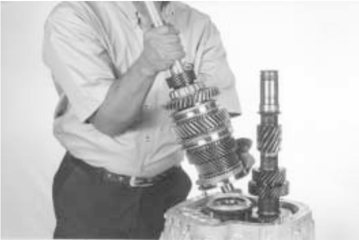
40.- Remove the mainshaft assembly, from the clutch housing, as shown.
