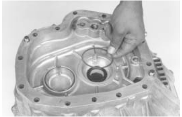
50.- Install the appropriate shims to achieve the proper end play, this total gives you a shim pack thickness to start the end play measurement.
