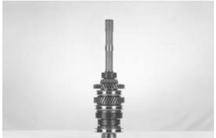
41.-Install the mainshaft assembly in a support or vise equipped with soft jaws or wood, shaft front facing up, as indicated.
