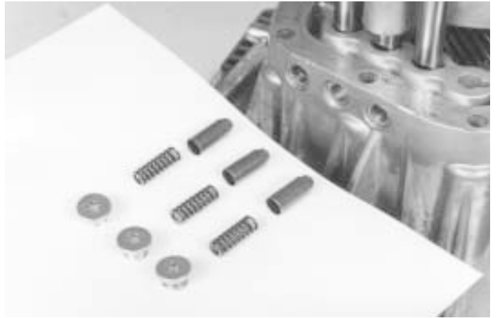
75.- Install the detents and detent springs, as indicated.
