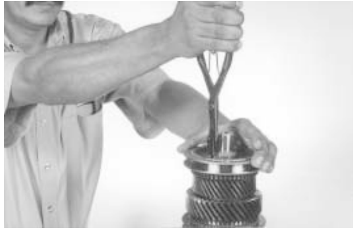
54.- With a snap ring plier, remove the hub snap ring, as indicated.
