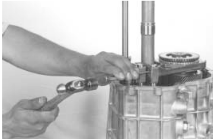
16.- Using a 5/32-inch drift and hammer, remove the pin from the fifth gear shift fork.
