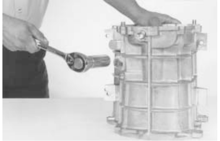
83.- Remove the reverse switch, as indicated.
