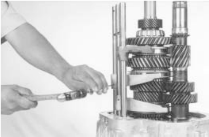
34.- Using a 5/32-inch drift and hammer, remove the split pin. From the 1st & 2nd fork and shift rail.
