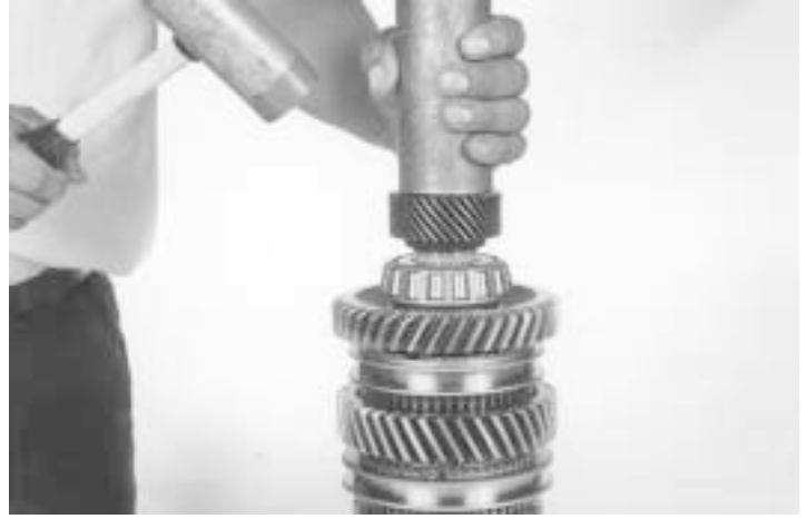
44.- Use a special tool or a press to install, as indicated.
