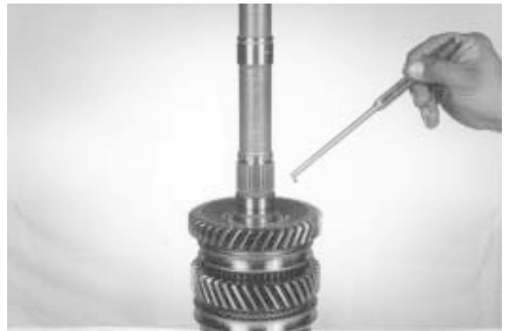
44.- Remove the locating ball, as shown.
