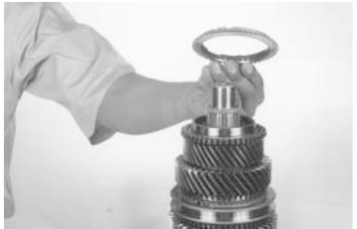
56.- Remove the 3 rd speed synchronizer blocking ring, as indicated.
