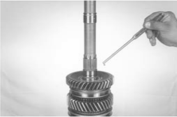
39.- Using a magnet, Install the ball, use grease to hold the ball in place.
