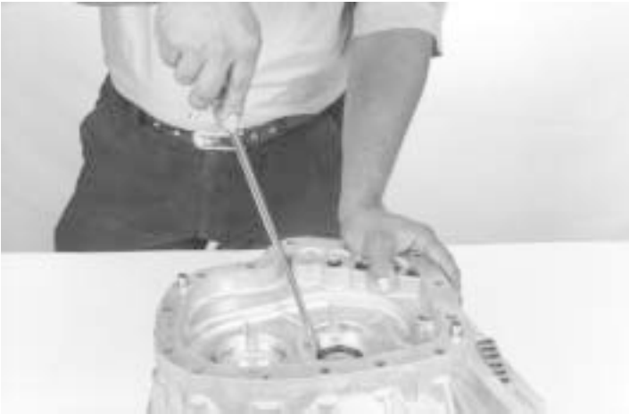
78.- Remove the input shaft seal, as shown.
