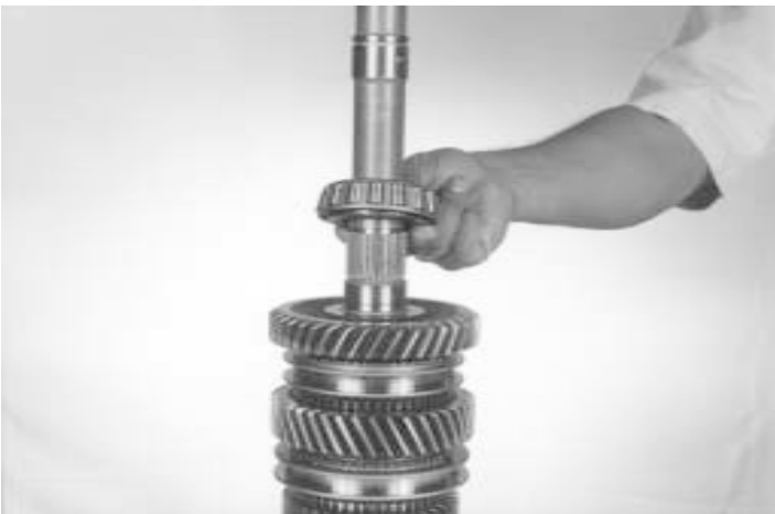
41.- Instal the bearing cone, as shown.
