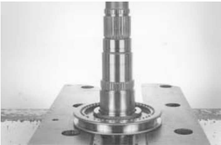
66.- Using a special tool or a press, remove the 3 rd & 4 th Synchronizer, as shown
