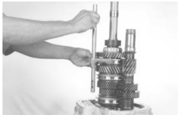
39.- Remove the reverse fork and rail as indicated.
