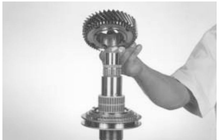
18.- Install the 2 nd speed gear, as indicated, rotate the gear to align gear slots with inner cone tabs.
