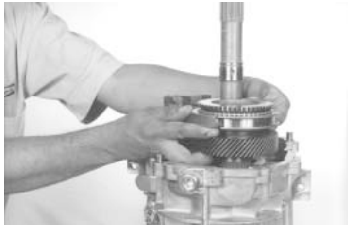
95.-Install the 5 th gear shift fork, the synchronizer assembly, the synchronizer cone and fifth gear as an assembly.
