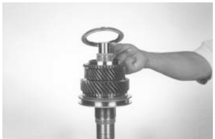
24 .- Install the 3 rd speed synchronizer blocking ring, as shown.
