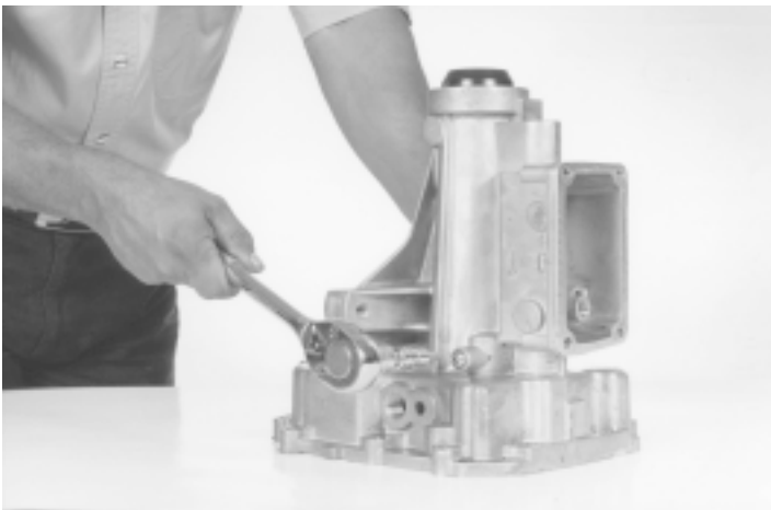
84.- Remove the fifth & reverse inhibitor bolt, as shown.
