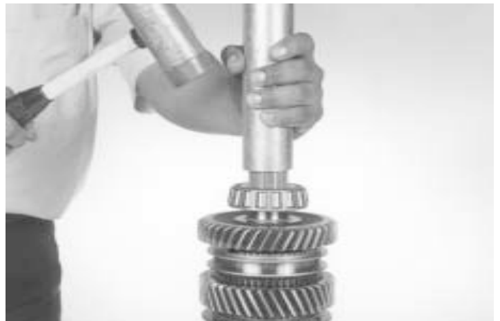
42.- Use a special tool or a press to install, as indicated.
