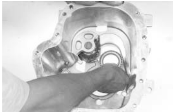
60.-Install the countershaft bearing cone, as shown.
