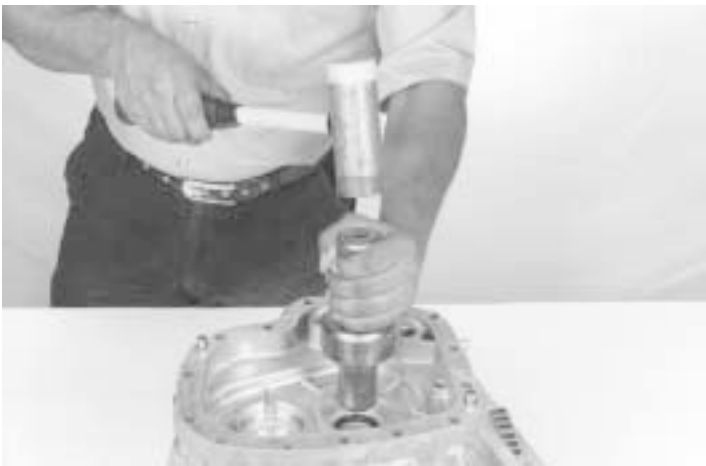
47.- Using a special tool, install the input shaft seal.
