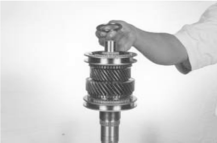
27.- Install the input shaft bearing race, as indicated.
