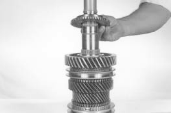
47.- Remove the clutch cone, as shown.
