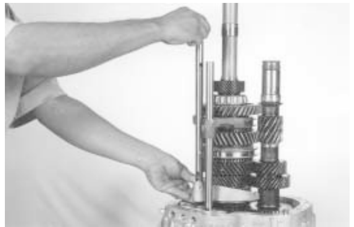
37.- Remove the 3 rd & 4th., fork and rail as indicated.
