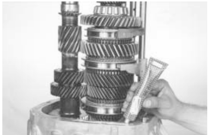
77.- Clean the mating surfaces of the transmission main case and the clutch housing. Apply a bead of silicone rubber to the sealing surface on the clutch housing then install the transmission main case.
