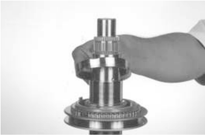
62.-Remove the second speed gear synchronizer inner cone, as shown.
