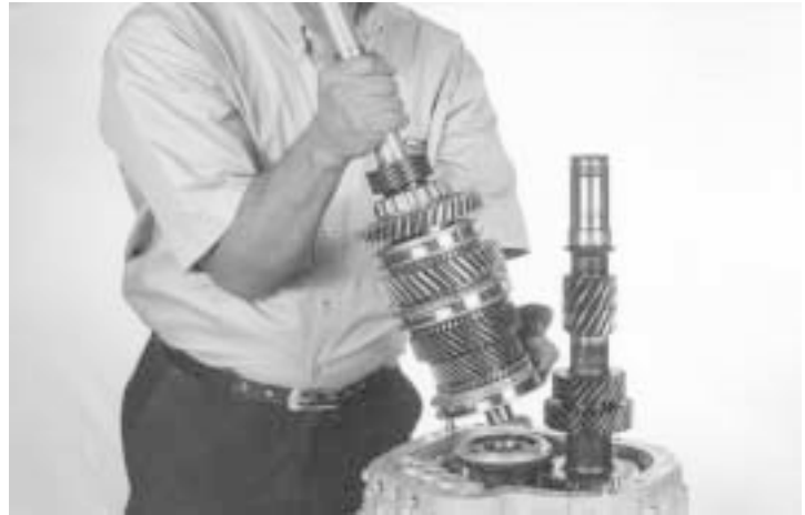
58.- Install the main shaft assembly, as shown.
