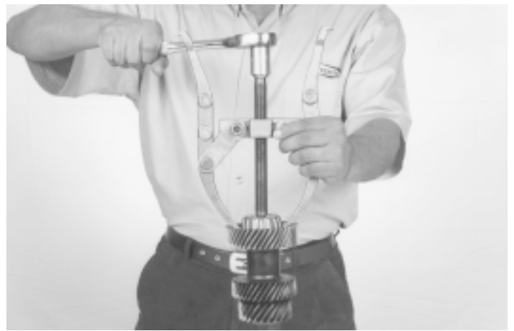
68.- Remove the cone bearing, as indicated.
