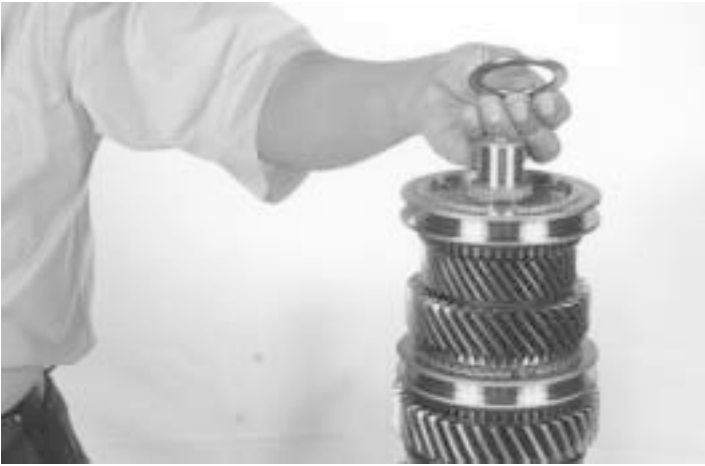
53.- Rotate the output shaft with the input end facing upward and remove the input shaft bearing race, as shown
