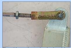
The cable attaches to the clutch pedal using a clevis/pedal bracket. The bracket mounts to the pedal with no modifications, and positions the cable at the highest point above the pedal pivot in order to maximize leverage and minimize pedal effort.
