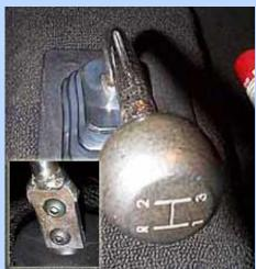
You can maintain the stock look by modifying the early shifter. We hacked off the 3spd/4spd lower bracked and welded on a metal tab. Drill two 3/8" holes to match the T5 shifter nub. Slip the stock boot over it and no one can tell from the inside that you've got an extra gear!
