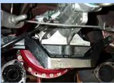
The <u>Modern Driveline</u> crossmember is a strong piece which follows the stock shape, making for better header and exhaust clearance.
