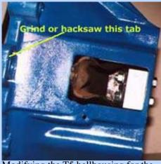
Modifying the T5 bellhousing for the early style clutch fork requires this 1" thick spacer block under the fulcrum to make up for the longer input shaft (hence deeper bellhousing.)
