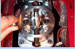
10 With the new shifter positioned over the studs, the nuts and washers are secured evenly.
