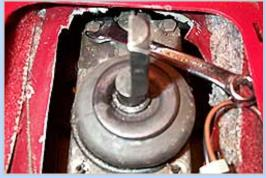
**3** With the dust boot removed and the swearing out of the way, we're ready to remove the shifter itself. Once again a sockets make easy work of the rear two bolts, but the front two require a wrench. **4** Note that our '88 was originally an AOD car which we converted to T5(hence the green shifter light and carved up transmission tunnel.)
