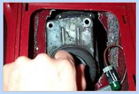
**5** With the four bolts removed, a little prying is all it takes to break the silicone bead holding the stock shifter to the T5.
