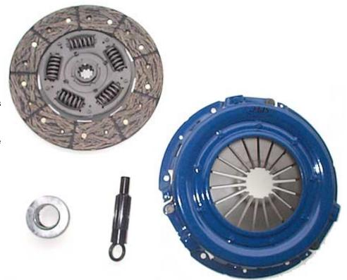
Selecting the proper clutch is a key ingredient of the T5 swap. You don't want to skimp here, otherwise you'll be doing the work all over again We talked to the clutch experts at SPEC (Star Performance Engineered Clutches), and they recommended their Stage 1 clutch, PN:SF481. Their stage 1 clutch will hold 300 horsepower with no problems, yet allow for chatterless engagement and low rpm driveability. At about \$159, including throwout bearing and alignment tool, the price is right too.
