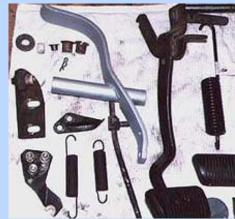
Converting an early Ford from automatic to manual requires rounding up the original clutch activation parts. This can be tough, the best bet is to find a wrecked four-speed car and take everything. Shown here are parts fro an early Mustang, including the z-bar
