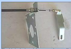
The kit is designed for strength as well as ease of installation. The 1/8" thick steel support plate mounts between the firewall and master cylinder. It not only locates the cable but strengthens the firewall by distributing the brake and clutch pedal loads.
