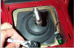
2 Getting the dust boot off is one of the frustrating parts of the otherwise simple installation. The two screws at the back can be reached with a 1/4" drive ratchet and 11/32" socket on an extension. However the two front screws are hidden under the console, and will require patient removal, half-turn at a time, with a open end wrench.
