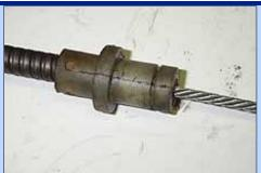
Stock cables, such as this 5.0L unit, use inferior nylon ends and a bare cable which eventually binds and corrodes. The lined cable included in the Modern Driveline kit offers a smooth and virtually frictionless pedal effort.
