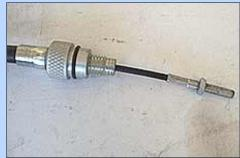
The cable is not an off-the-shelf stock piece as found in some conversion kits, it is a custom spec'd piece with a duel-lined inner cable and an integrated firewall tension adjuster.
