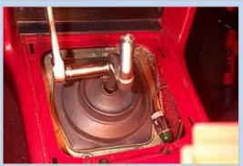
1 Installation is about an hour long task. With the knob, leather boot and cover plate removed, we used a 1/2" socket to remove the stick from the shifter. Notice we'd been using an aftermarket stick with our stock shifter in attempts to shorten the throw.
