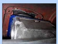
Slight clearancing of the shifter opening in early may be required. We had to do it on our '67 Mustang, but in a '65 the T5 lined up perfectly.
