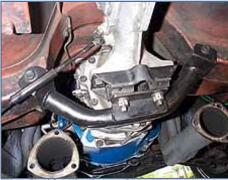
The California Pony Cars T5 crossmember serves its purpose, however the mount bracket welded to the main tube is a weakness. The member also offers less exhaust clearance.
